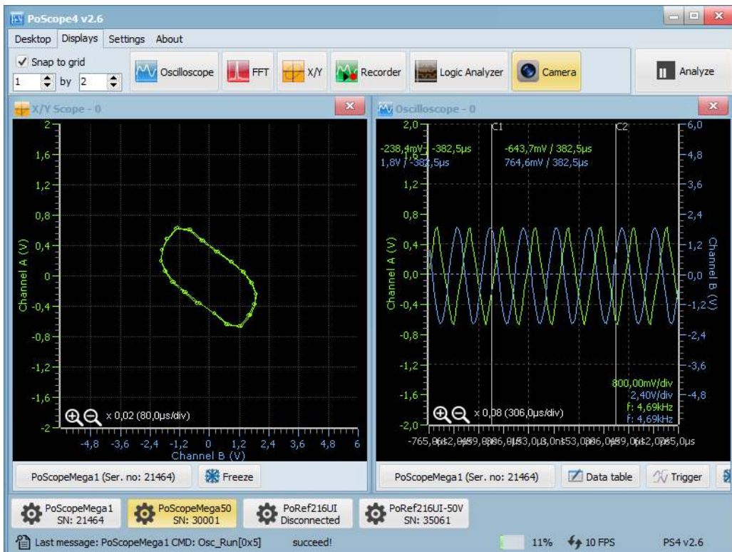
Channel A is triangle and Channel B is sine
