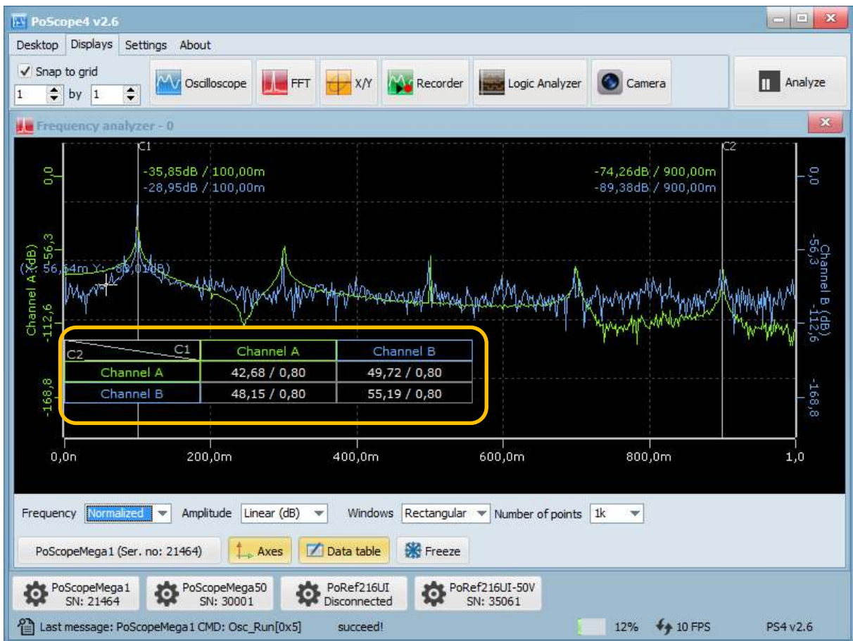
Frequency analyzer with data table open
