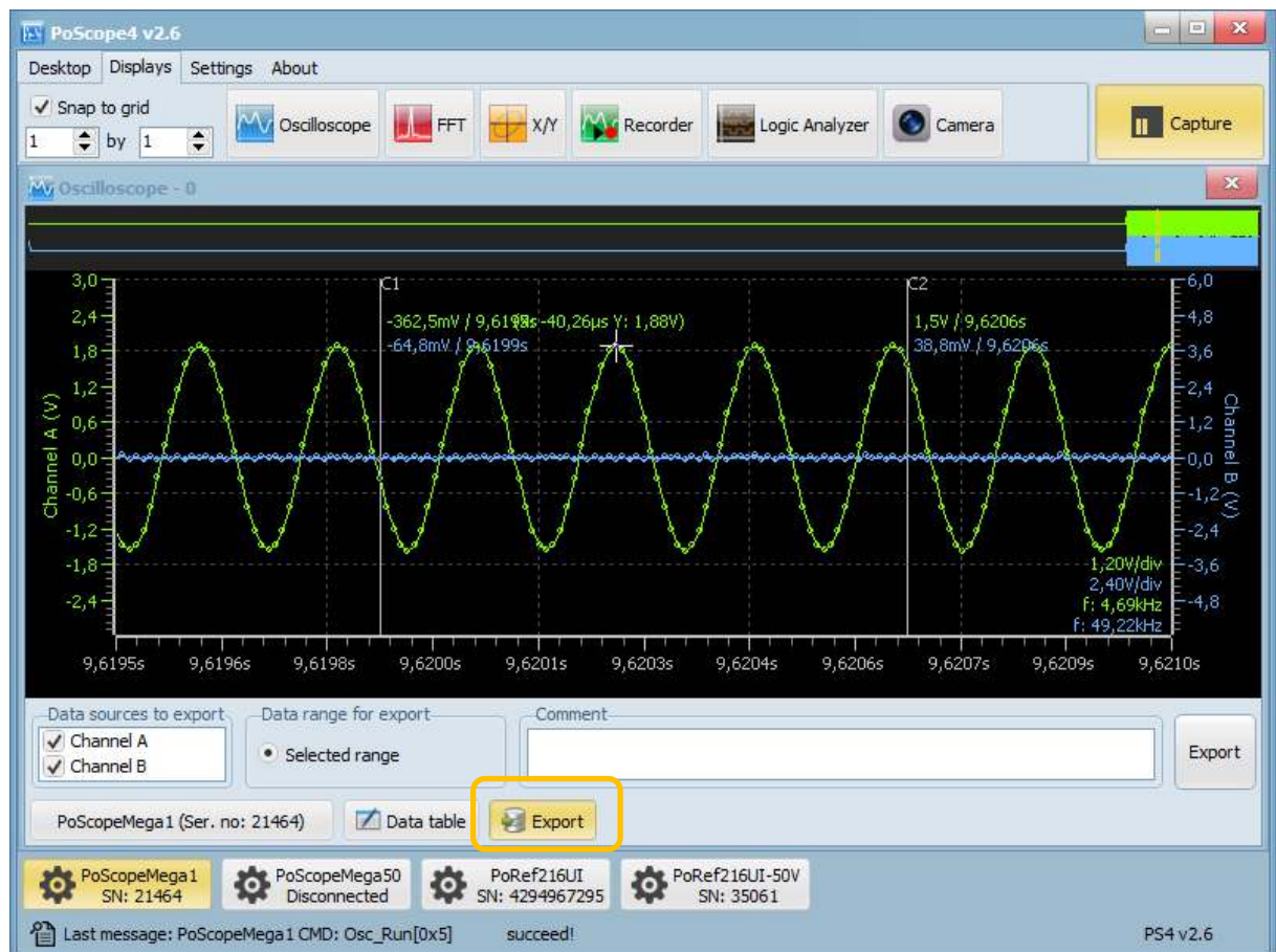
Oscilloscope display in Analyze mode with export settings
