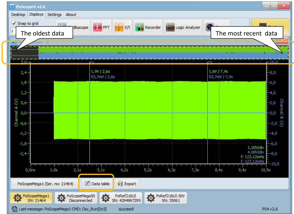
Oscilloscope display in analyze mode with Overview window
