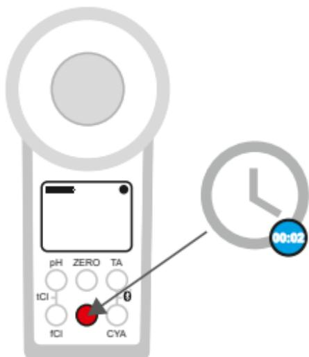
On/Off button can also be used to skip countdown during measurement (not recommended)
