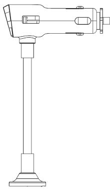
Alternatively you can use the USB charger, included in delivery content. In this case, please plug in the USB charger in the power supply socket in your car. Connect the other side of cable with the Micro USB plug of DABMAN 61 plus. [please see point 9, chapter 4] and use the magnetic holder [please see chapter 3] for fixing in air vent of the car.
