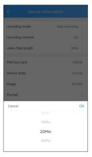
In this setting you can see the SD card information like Storage capacity, Status and used Space. For format the SD Card, Tap "Format". There will be confirmation pop-up. Tap "OK".
