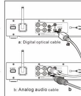
Use an RCA audio cable or optical cable to connect the DVD player / TV outputs with the AUX / OPTICAL input socket from the device.
