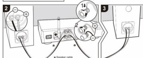
After inserting the speaker cables, tighten the terminals firmly by turning to the right. Also make sure the exposed wires of the speakers do not stick out of the speaker terminals when connecting. If the exposed wires of the speakers touch the rear panel or the i and s wires touch each other, the protection circuit may be activated and the power may turn off.
