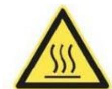
Please do not touch surface while in use. The temperature of accessible surfaces may be high when the appliance is operating.
