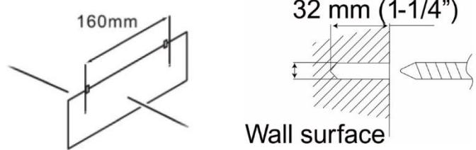
Attach the screws with proper dowels as you can see in the pictures
