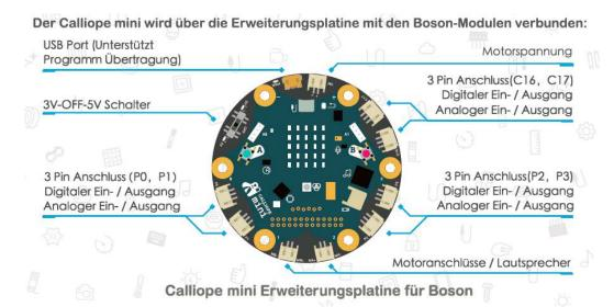
The Calliope mini expansion board for Boson is used to hook up Boson modules to Calliope mini board. The expansion board comes with an edge connector, 6 fool-proof 3-Pin sockets, 2x PH2.0-2P motor driver ports and switchable 3.3V/5V power system. We can change the power if you need more power to drive servos. Moreover, to upload the program conveniently, the USB port on expansion board can support program and power together.
