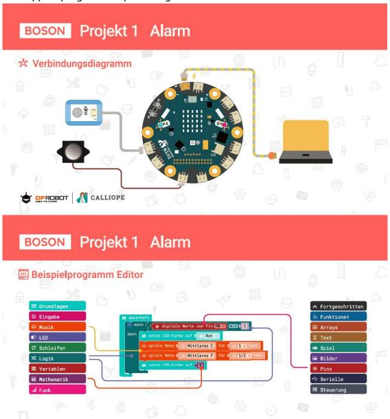
To help you easily understand the usage of each module, the boson kit for Calliope mini is provided with a quick start guide, including 5 basic projects with wiring and sample codes. Walk through the guide and create your own invention!
