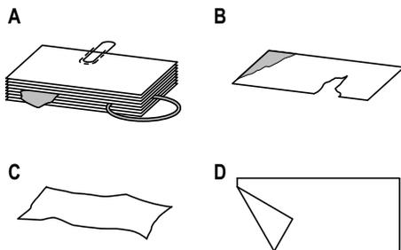
➔ Check the batch of bank notes for paper clippings, paper clips, rubber bands and other foreign bodies and remove them before inserting the bundle in the machine (Figure A).
