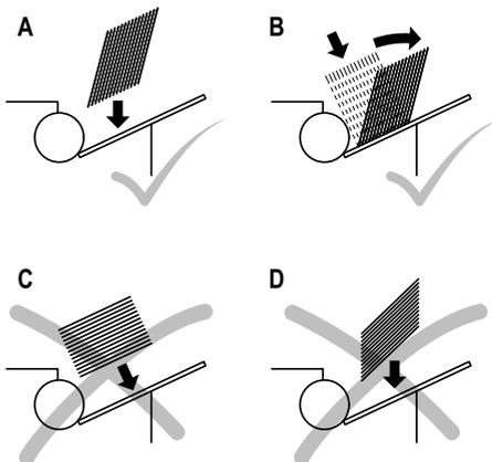
➔ Slide and fan the bank notes in the batch so that the top bank note is somewhat lower than the one following. Insert the bank notes in the infeed tray [4] (Figure A).
