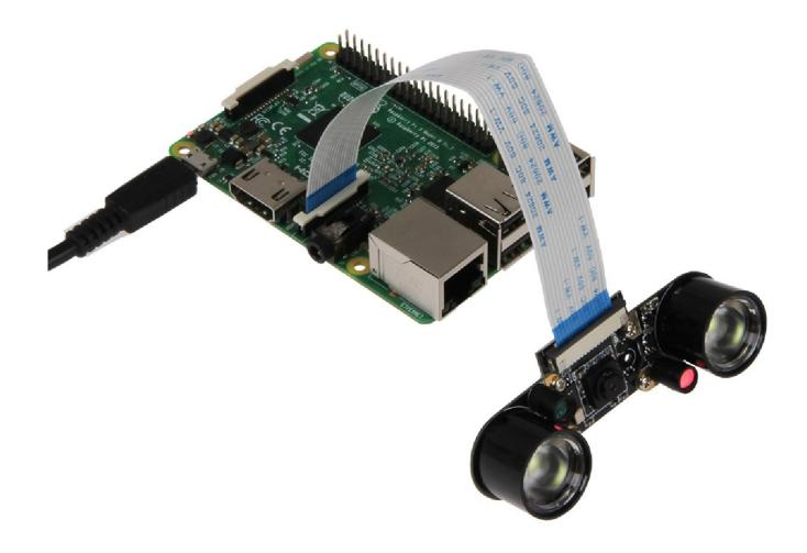
Connect the camera module, as seen in the image, with the shipped ribbon cable to the CSI interface of your Raspberry Pi.
