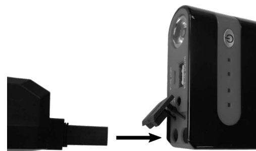
Figure 2: Connecting the jumper cable
