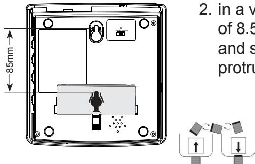
2. in a vertical line, drill 2 holes at a distance of 8.5 cm from each other and insert plugs and screws; let the head of the screws protrude for 5 mm
