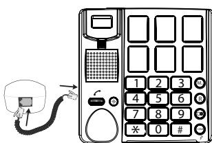
1. connect the receiver with the telephone by attaching one side of the spiral cable to the bottom of the receiver and the other side to the left side of the telephone
