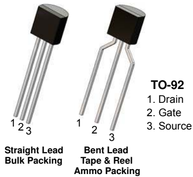
Figure 1. J175 / J176 Device Package
