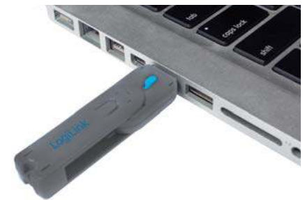
Insert the Key with blocker to an USB port
