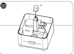
\*The cover prevents water flowing into the air outlet U)
