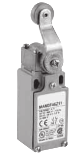
Rollenhebel MAM1F45*** F45: Nylonrolle F46: Metallrolle
