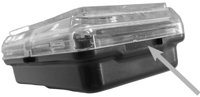
Figure 3: Lifting off the cover glass
