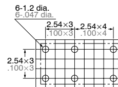
PC board pattern (Copper-side view) Single side stable 2 coil latching
